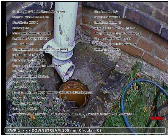
20191023-085610-snap0000.jpg, 00:00:03, 0.00 m Start node type, gully, reference number: 1
